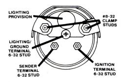
When connected, as shown, the pointers move when current (power) is applied. All instruments also deliver proof of operability.
